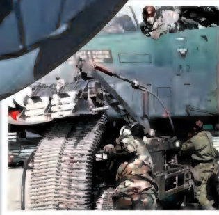
Left: 30mm rounds loaded into an A-10A Thunderbolt II
